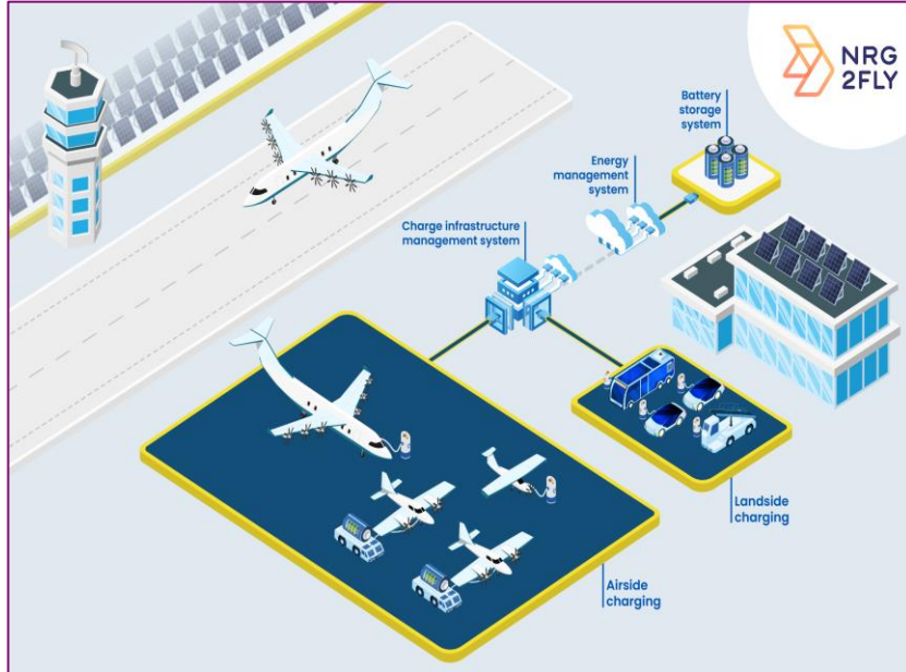
Airport electric infrastructure (source: NRG2FLY)
